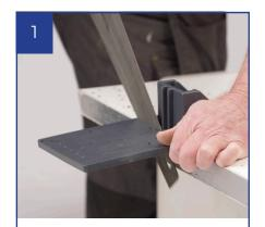
Firstly, cut the limpet base plate in half with a wood saw, and dispose of the adjustable bracket section.
