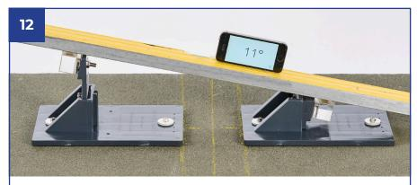
With the rails fitted to the angled sides of each bracket & the adjustable vertical bracket extended fully and locked in place, the PV panels when clamped to the rails achieve a 10-11° pitch.
