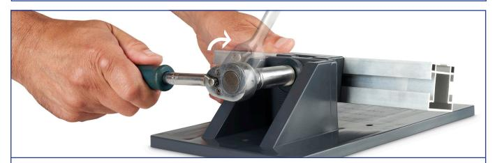
When fixing the rail to the Adjustable Bracket and the Flat Roof Bracket, tightening until the nut bites & then another quarter to one third turn is sufficient.
