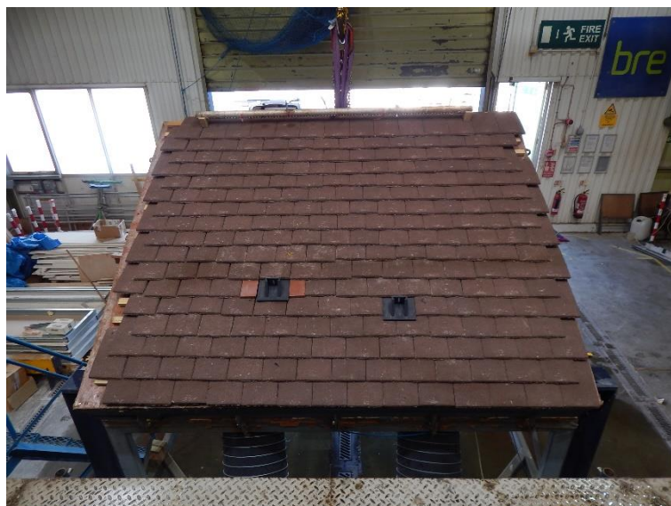
Figure 10 Test set up for Rosemary plain tiles.
