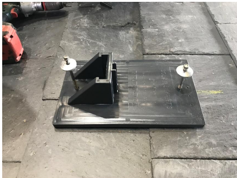
Figure 12 Image to highlight the test set up for the brackets with slates.
