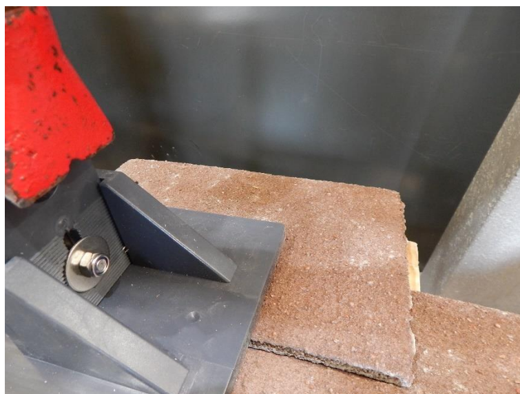
Figure 20 The bracket on plain tile under test.
