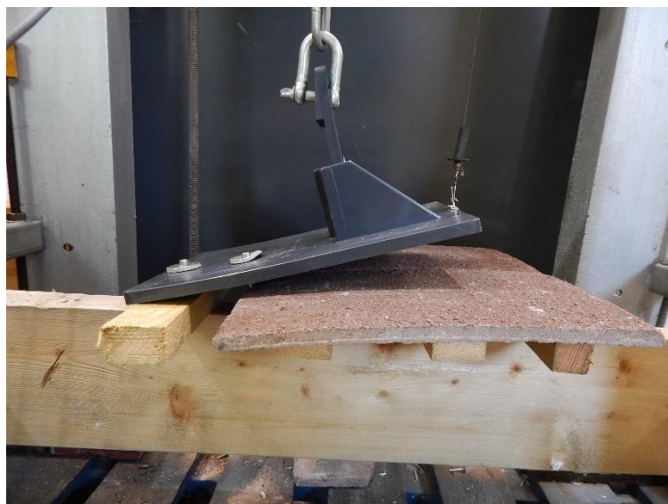
Figure 15 The bracket on plain tile under test at failure.
