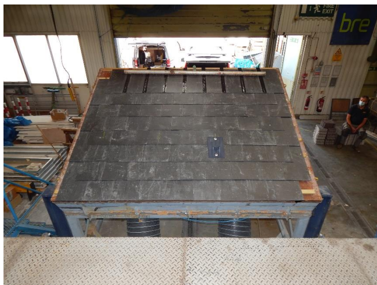
Figure 13 Test set up for PV brackets with slates.
