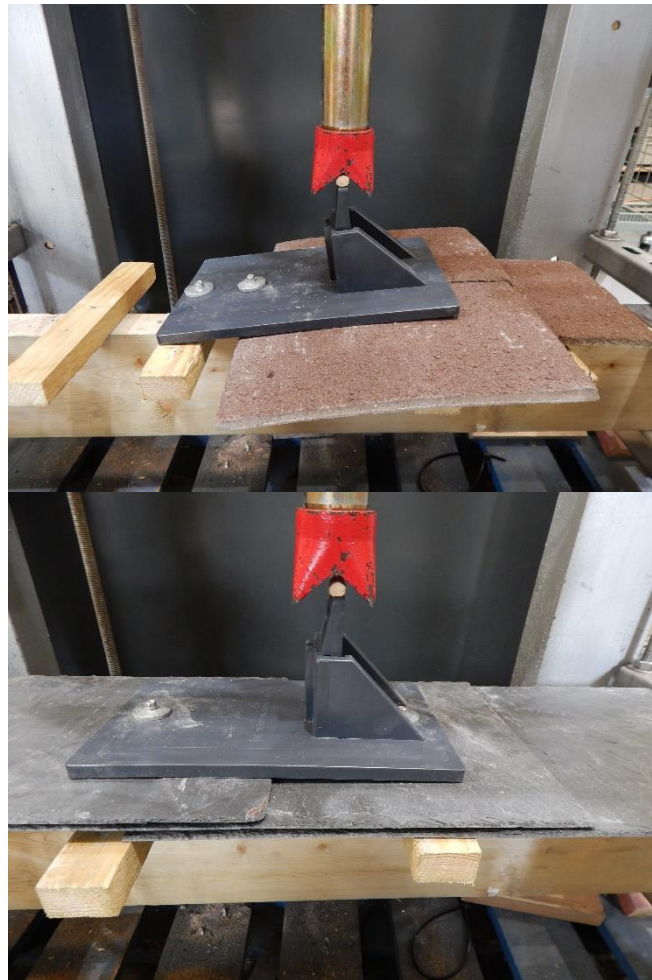
Figure 14 Test set up for positive load test (plain tiles top, slate bottom).
