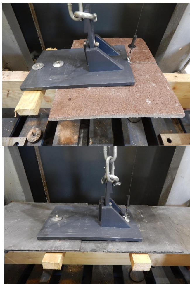
Figure 3 Example of the setup of the test rig with rafter, roofing element and bracket (plain tile top, slate bottom).
